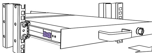
6. Pull rail-release switch and pull console out. (Both sides. Be careful when pull out console.)
