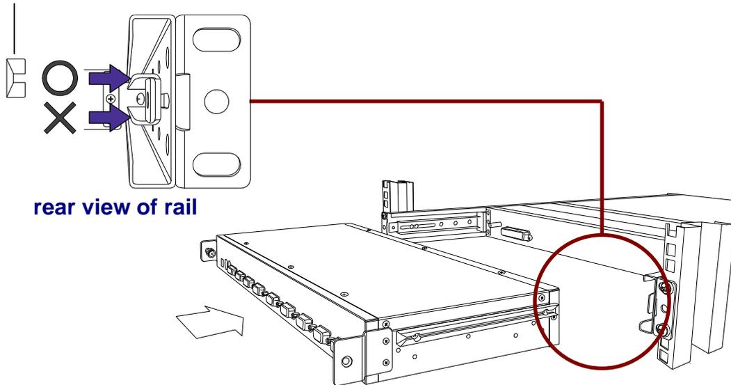
3. Tight thumb screw of bracket up to fix KVM switch in console and finish installation. (Both sides)
