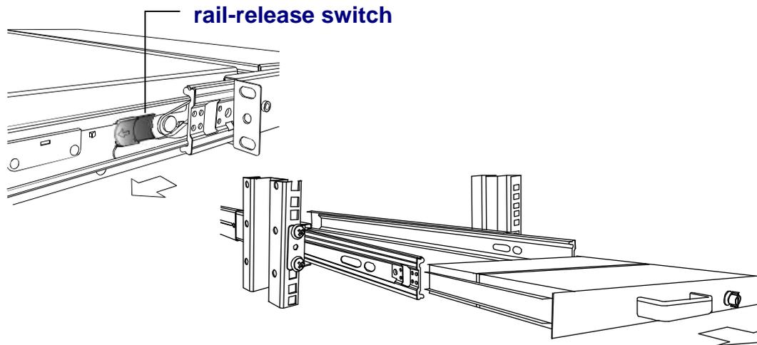
7. Push rail-lock switch on the rail and push rail back. (Both sides)
