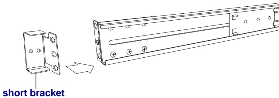
4. Install four screws (don't tight-up) to combine rail, short bracket and bracket attachment.
