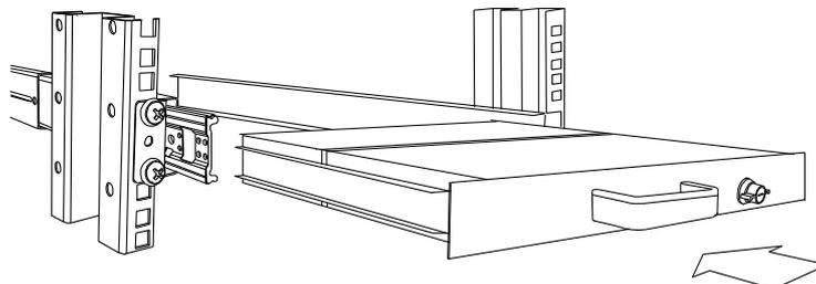
8. Unlock and pull rail-lock switch (left and right at the same time) then push console to the end.
