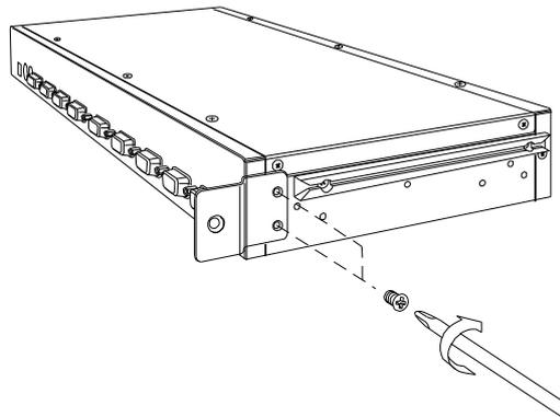
2. Push KVM switch into the rails from rear of cabinet.
