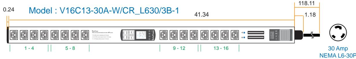
Cordset : 3 meter UL 10AWG cable with 30 Amp NEMA L6-30P plug
