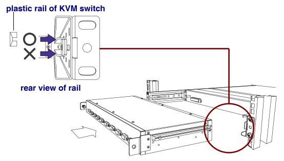
3. Tight thumb screw of bracket A up to fix KVM switch in console (Both sides) and finish installation.
