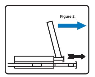
Pull and hold the black arrow button on either side of the LCD console drawer to unlock. (shown in Figure 2).
